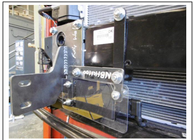
Figure 6: Adjust sonar bracket to be parallel with the radiators and vertical.
